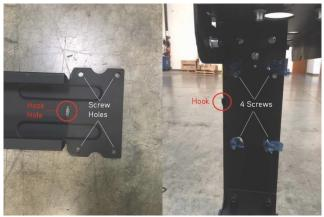
Un-screw four screws on each side of stand (8 total) and attach second support beam by lining up hook with hook hole. Once the support beam hook is inserted, screw in four screws on each side to attach support beam.
