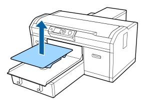
4. Check the installed spacers and determine which spacers you need based on the platen and fabric you are using.
