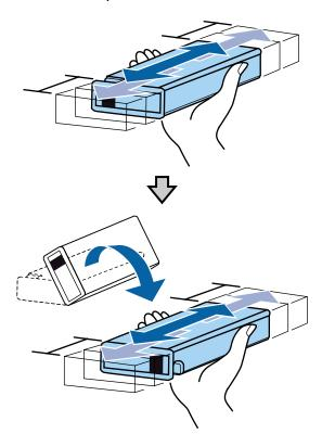
**Caution:** Do not touch the IC chip on the end of the cartridge; otherwise, the cartridge may not be recognized, or the printer may not print properly.
