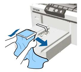
7. Tuck the sleeve around and under the frame so that it does not drape over the movable base.
