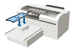
2. Pass the fixing band under the parallel adjustment plate and align it with the groove on top of the platen and secure it tightly. Make sure the end of the fixing band is on the side of the platen.
