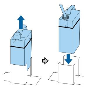
**Caution:** Verify that the waste ink tube is still inserted into the neck of the bottle. If the waste ink tube comes out of the bottle, waste ink will spill out.
