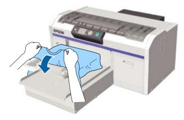
4. Gently pull the T-shirt over the edges of the platen to flatten it.
