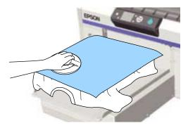
**Note:** The printer detects the highest part of the garment surface. If there are any wrinkles, creases, or slack, a platen height error may occur or print quality may decline. Stretch the T-shirt to remove the slack, however, do not stretch the T-shirt so much that the printed image will be distorted.
