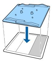
3. Flip the platen over and rub the section of the grip pad where you removed the backing to adhere it to the platen.
