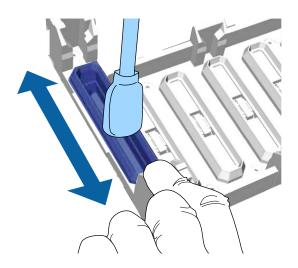
10. If necessary, remove any excess ink from the edges of the cap.
