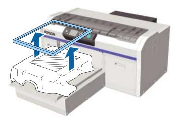
2. Hold the T-shirt by the shoulders and carefully remove it from the platen; the ink is still wet and can be easily smudged.
