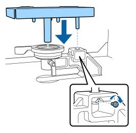
12. Rotate the fixing lever as shown to tighten it and secure the height adjustment lever.
