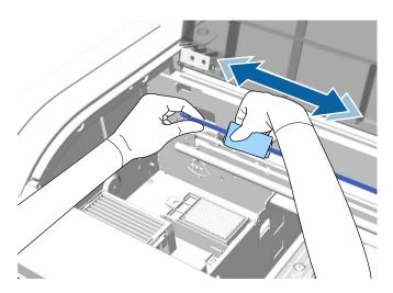
**Caution:** Do not pull on or rub the encoder strip (carriage scale) with too much force, or the right side may detach or the encoder strip (carriage scale) may be damaged, causing the printer to operate incorrectly.
