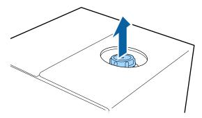
**Note:** Make sure you pull the cap section out of the hole in the cardboard. If the cap is opened without being pulled out, the pre-treatment solution may spill out.
