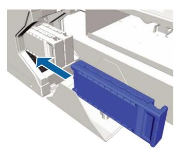
**Note:** Do not touch the IC chip on the top of the cartridge; otherwise, the cartridge may not be recognized, or the printer may not print properly.
