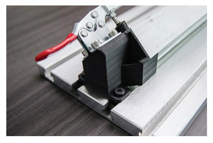
Every manufacturing company in every industry has a need for fixtures; either for assembly or inspection. They come in all shapes and sizes depending upon the market, but their common purpose is to hold a part in an exact, mistake-proof orientation while another operation is performed on it by a worker or another machine.
