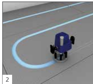
2 Cut grooves using the router. Cutting width should be the same as the pipe width; cutting depth should be at least 3 mm deeper.
