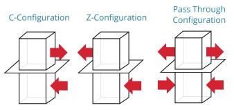
The Lift Configuration refers to the unloading and loading pattern of the lift. This lift allows for loading and unloading on the same side ("C"), from front to rear ("Z") or pass through.
