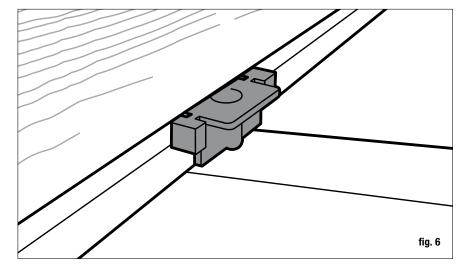
Note: To predrill a groove on one side of deck board, we recommend using a 4mm T-slot cutter.
