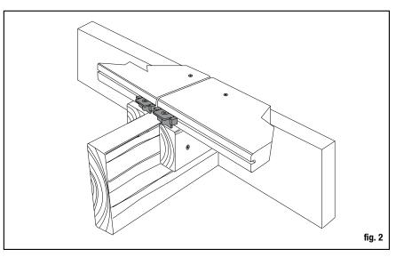
Fasten the outside edge of the first board to the rim joist with screws. Pre-drill and countersink all deck screws, regardless of type, that are within 38mm of the end of the deck board. On the other side of the board, place a Stowaway hidden fastener into the slot and center on the joist.
