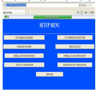
By selecting the "Edit Marquee Messages" button, the user can set up the message text, font size, color, and functionality of the message to be displayed on the marquee sign.
