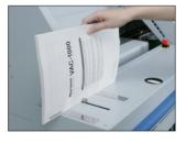
Book thickness is automatically measured by placing the book block into the digital caliper. Thickness data automatically begins set-up of the clamp, milling and adhesive application stations, nipper opening and cover scoring. This provides operating efficiency for short-run book production.
