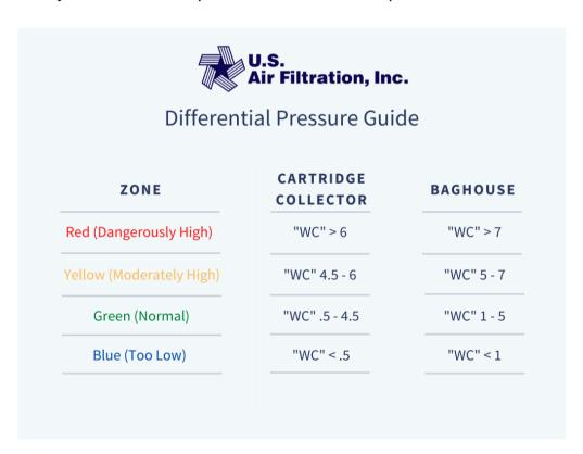
[ ] If your differential pressure is in the blue range noted above, perform a leak detection test.
