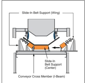
The track upon which idlers slide can be incorporated into the design of the conveyor as part of the structure.
