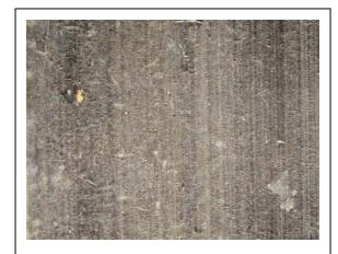
Abrasion from material loading will be seen as wear in the top cover in the load carrying area of the belt.
