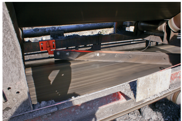
Diagonal plows are installed across the belt at an angle of 45 degrees to the direction of travel.
