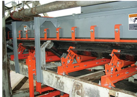
When two or more cradles are installed, the use of intermediate idlers idlers placed between the adjacent cradles is recommended.
