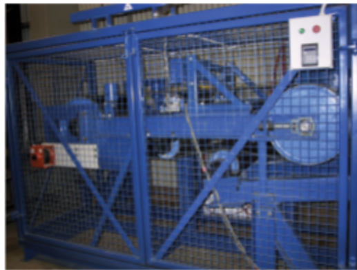
A barrier guard is a fence, or other obstacle, to keep personnel away from a conveyor and its components.
