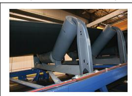
An idler consists of one or more rollers, each with one or more bearings. The rollers are supported by, or suspended from, a framework installed across the conveyor stringers.
