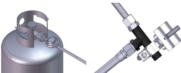
Propane tank: height = 456mm, diameter = 320mm
