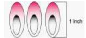
Visually check the burner flames prior to each use. The flames should look like picture, if they do not, refer to the cleaning burner tubes and ports, see page 14 of this manual.
