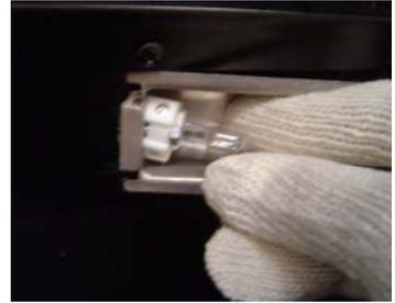
8. Replace glass cover, reinsert light bulb housing into the grill, and insert and tighten all the screws. Picture G.
