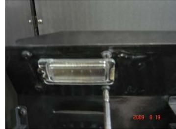
9. Attach original lamp rear cover with original 8pcs screws and washers to back panel of firebox and tighten screws as Picture H.
