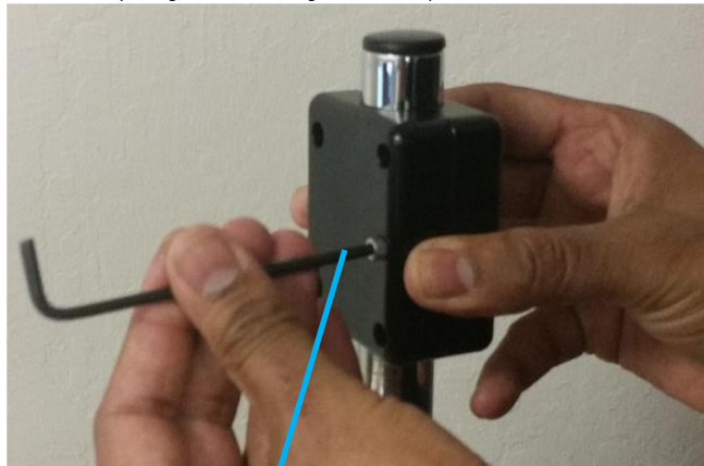
Tighten with Allen Key (5/32")
