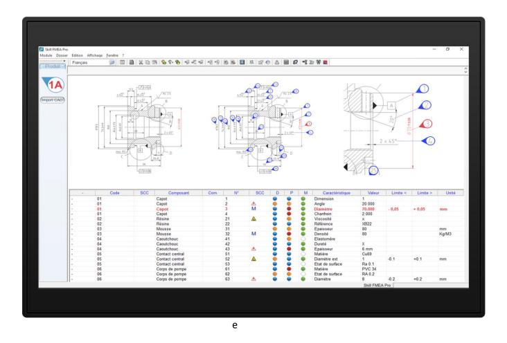
**ONE DIMENSION, ONE PICTURE**: The all list has been integrated into the Skill FMEA Pro software with one picture for each dimension. Integration of the component into the FMEA = one click!
