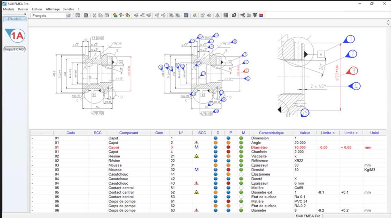
The screenshot displays the Skill FMEA Pro interface. On the left, a sidebar shows 'Produit' and 'Import CAD'. The main area contains three CAD drawings of a mechanical part with dimension callouts numbered 1 through 25. Below the drawings is an AMDEC table with the following columns: Code, SCC, Composant, Com., N°, SCC, D, P, M, Caractéristique, Valeur, Limite <, Limite >, and Unité.
