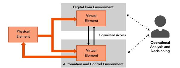
In newer deployments, the DT may share a common environment with existing automation and control systems (see diagram below)
