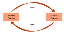
Recommendations of changes for optimal performance could be computed in the Virtual Element, and those changes sent back (in the form of control data), to the Physical Element.
