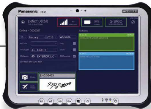
The "Defect Details" screen from Conduce Group's system on a Panasonic Toughpad.
