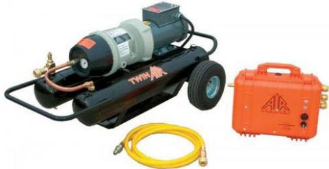
This compressor system is designed to provide automatic back-up air for up to 3 workers in the event of compressor failure. The COMP-3EA™ Compressor System includes an Auto-Air™ Breather Box®, model BB30-COAA, the TA-3EA compressor supplied with a CGA-347 high pressure reducing regulator, and primary / secondary hoses. An optional 60 or 87 cf cylinder can be installed on the compressor frame to provide additional egress air. The COMP-3EA™ system is designed for pressure demand respirators only.
