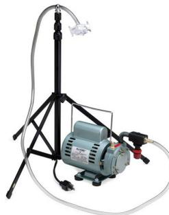
Lightweight and low maintenance, this rotary vane sampler has a sampling range of 0-30 LPM and is an excellent resource for sampling asbestos (25mm cassettes), lead (37mm cassettes) and mold. This sampler is the best value in the market today, meets OSHA and AHERA standards and comes complete with six feet of vinyl tubing, inline filters, rubber feet, for stability, handle and built-in switch. Optional adjustment aluminum stand. Weight 10 lbs.
