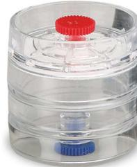
This 37mm, MCE cassette is .8µm mixed cellulose ester and is specifically designed for lead sampling. 50 per box. The cassettes are designed and manufactured to meet all applicable NIOSH/EPA/OSHA Standards for lead sampling. Each cassette is individually assembled, preloaded, flow tested, and marked under stringent quality assurance procedures.
