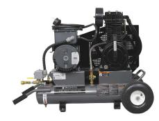
The heavy-duty AIRE-SWEEP® C17-185E Portable Air Compressor is powered by a 5 HP, 230 volt/30 amp electric motor. The C17-185E is designed for indoor use when a gas engine is impractical. The unit produces an outstanding airflow rate of 17.5 cfm at a rated pressure of 185 psi.
