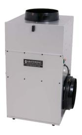
The larger CAP®1200-UV model has about 50% more air filtration capacity than the CAP®600UV. It features an additional 2"-deep particle pre-filter, a heavier duty VAPOR-LOCK® carbon filter, and a higher capacity HEPA filter, for added dirt holding and odor removal capacity.
