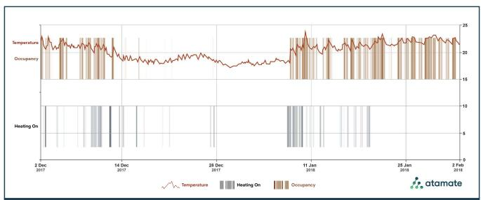
Figure 13: Occupancy-based electrical heating under atBOS controls in a single bedroom, showing the temperature dropping during a prolonged absence for the Christmas holidays but rapidly returning to the 21°C setpoint when the occupant returned.<sup>32</sup>
