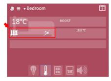
Heating is best controlled by presets explained below, especially if it involves underfloor heating or radiators that take time to warm up.
