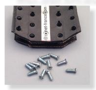
The SUPER-SCREW<sup>®</sup> is part rubber and part metal--a truly hybrid splice with the advantages of vulcanization and the quick and easy installation of metal. Material will not sift through the splice area as SUPER-SCREW<sup>®</sup> is a one piece construction without a hinge or pin. It's designed to reach from the end of the belt deep into the fabric for added strength and follow belt movement around pulleys, including "S" drives and gravity takeups.
