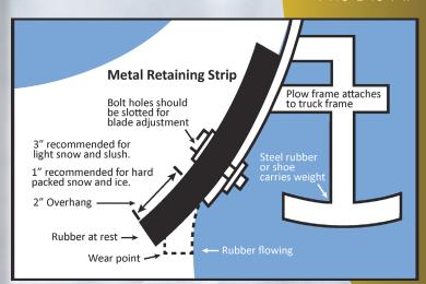
GREATER IMPACT ABSORBTION = REDUCED EQUIPMENT SHOCK = LESS FATIGUE/WEAR ON PLOW
