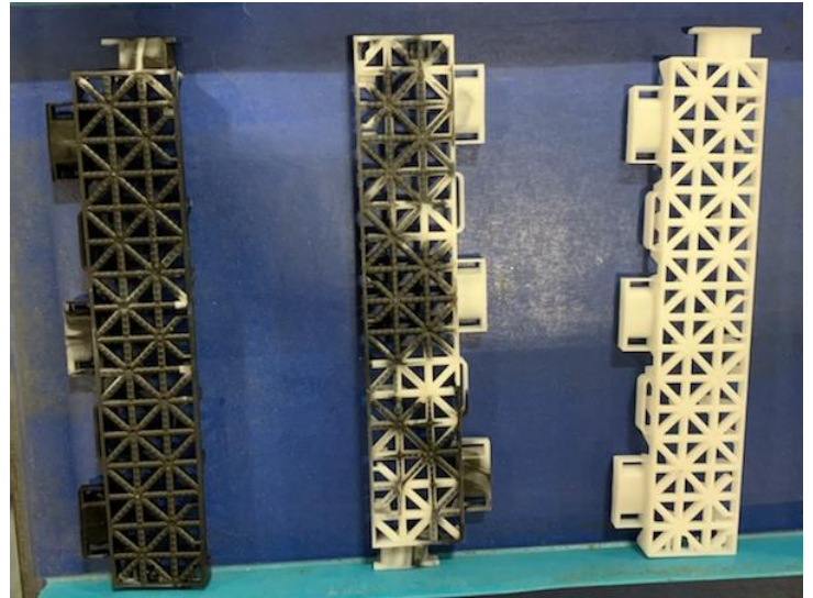
Above: Parts from an on-the-fly color change using Asaclean PLUS through our customer’s multi-cavity hot runners.
