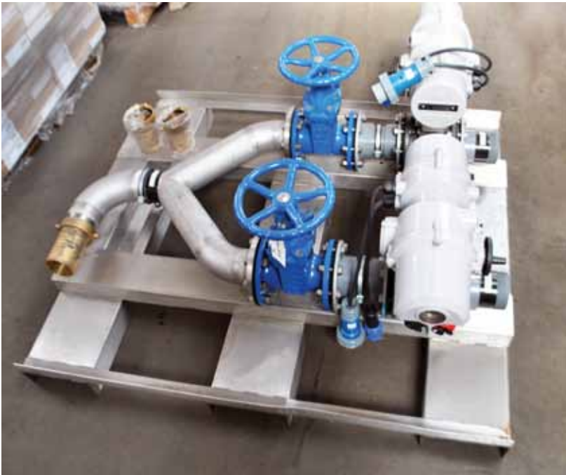
Twin Set of Rotork Automatic Actuating Control Valves
