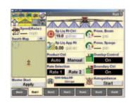
If the tank is to be drained, press the screen inside the container's bar graph area and select from the on-screen options as shown below.
