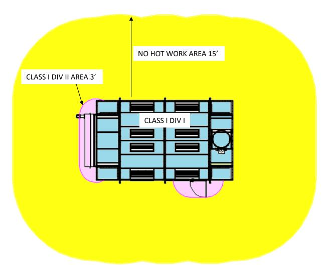
RESTRICTED HOT WORK AREA WITHING 15' ALL DIRECTIONS CLASS I DIV II WITHIN 3' OF ANY OPENING CLASS I DIV I WITHIN ENCLOSURE & EXHAUST DUCT WORK
