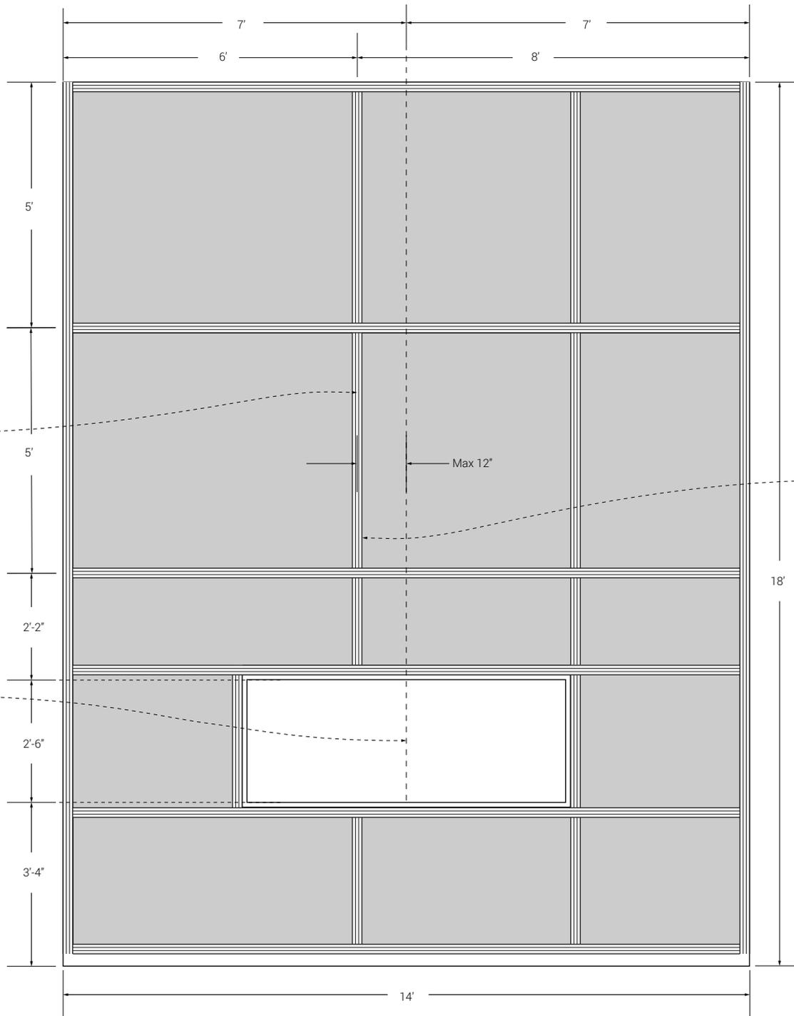
Make sure ENTIRE joint assembly is no more than 1' off centerline. Do not position such that any piece of Reveal™ Trim piece is more than 1' off centerline of window.
