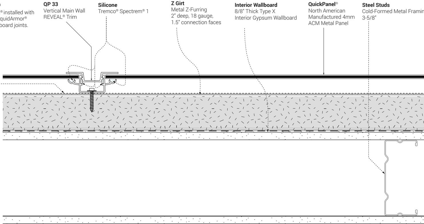
**1A** HEADER & FLASHING DETAIL
