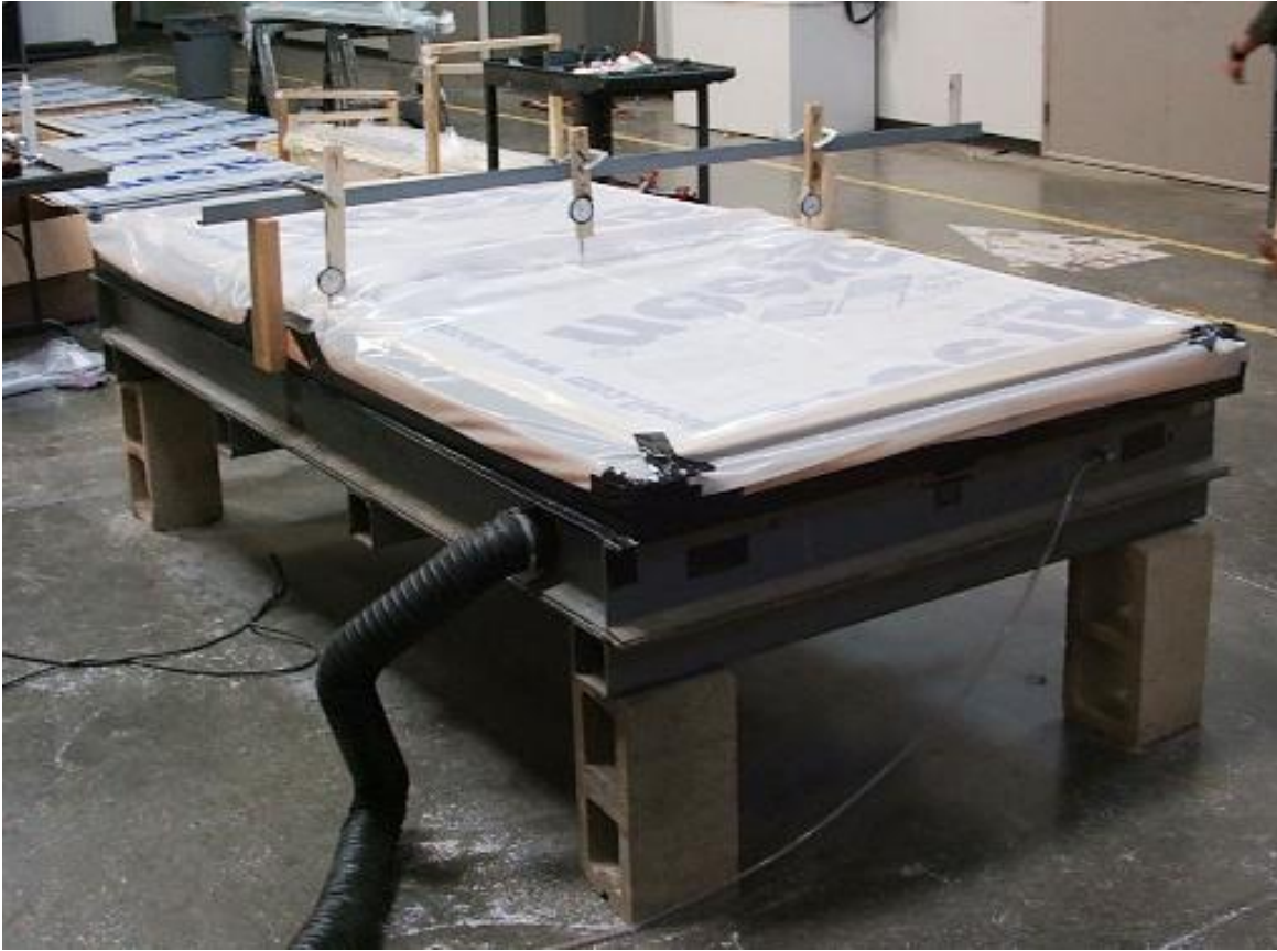
Photograph No.6 Positive Uniform Load Test Set-up
