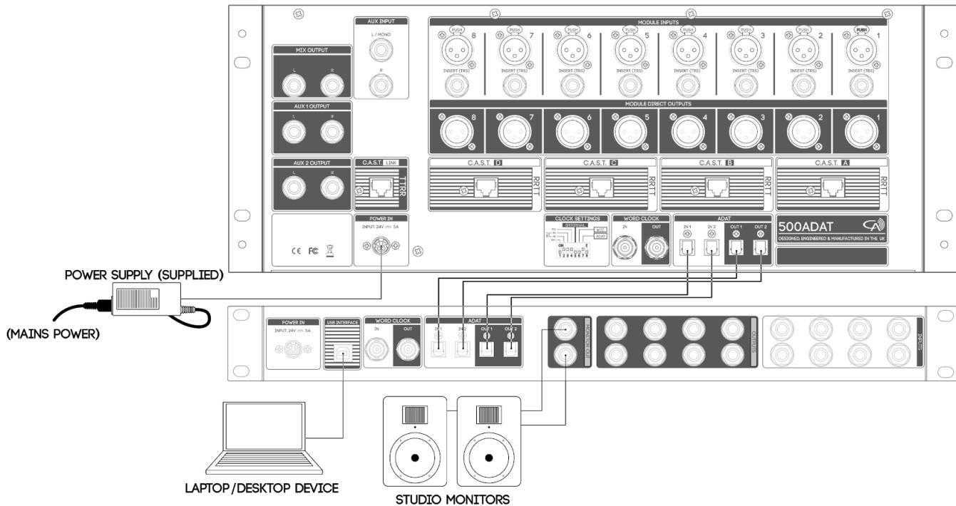
This hardware setup diagram will get 500ADAT connected to your audio interface and ready for recording.
