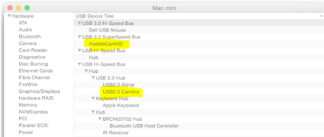
In this example, you can see the HuddleCam model in use connected as a fully functional USB 2.0 device (HuddleCamHD).
