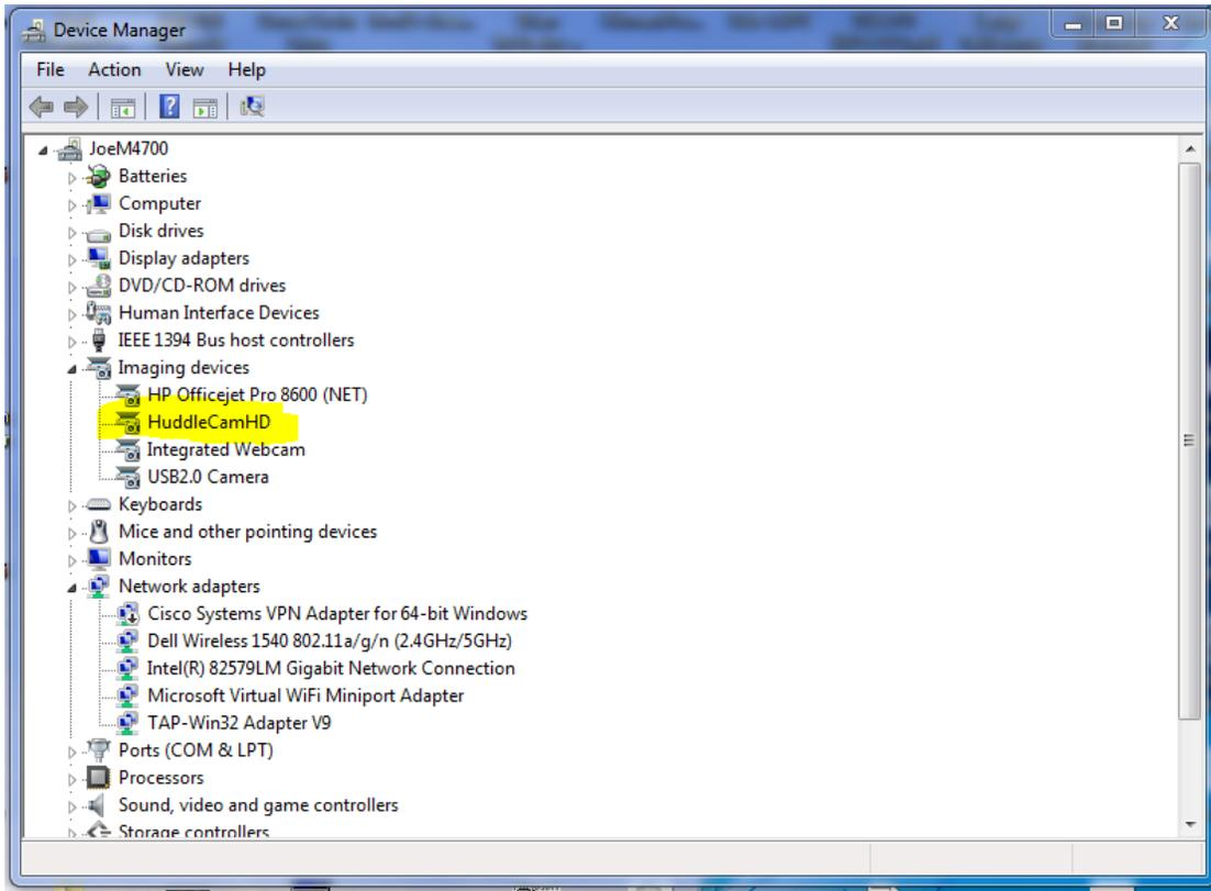
In this example, you can see the HuddleCam model in use connected as a fully functional USB 2.0 device (HuddleCamHD).
