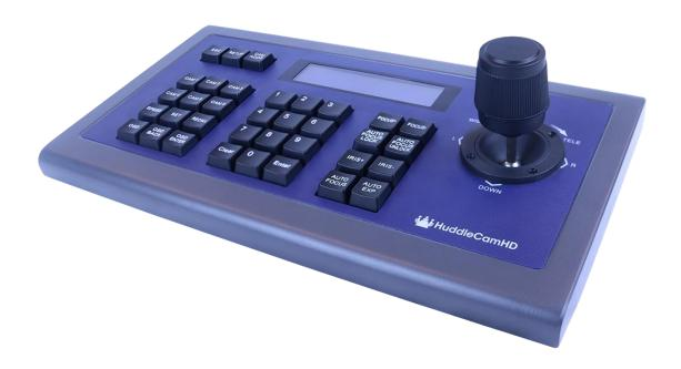
Easy pan, tilt & zoom controls for any RS-232, RS485, RS422 VISCA, Pelco-P or Pelco-D protocol camera!
