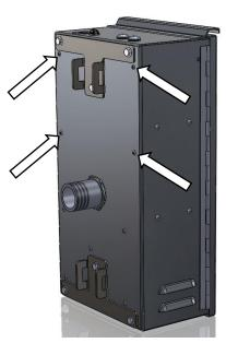
a. Current G Series cabinets will have four mounting screws on the right-hand side to remove.
