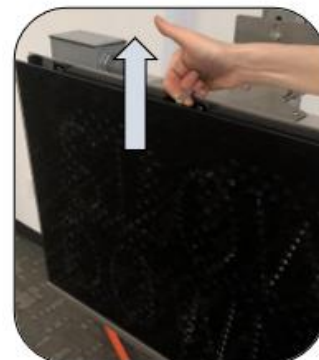
Lift window retainer clip
