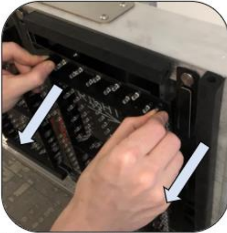
Being very careful not to touch the LED lamps, grasp the circuit board stiffeners at the top.
