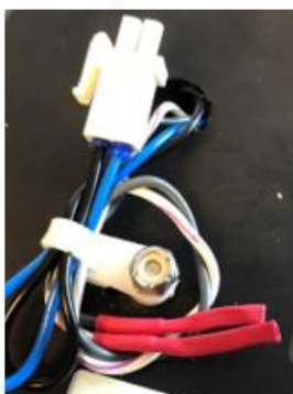
Optional: If present, disconnect strobe connectors.
