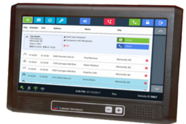
TCH - Transit Control Head - A Mobile data terminal that interfaces with IVN-R.
