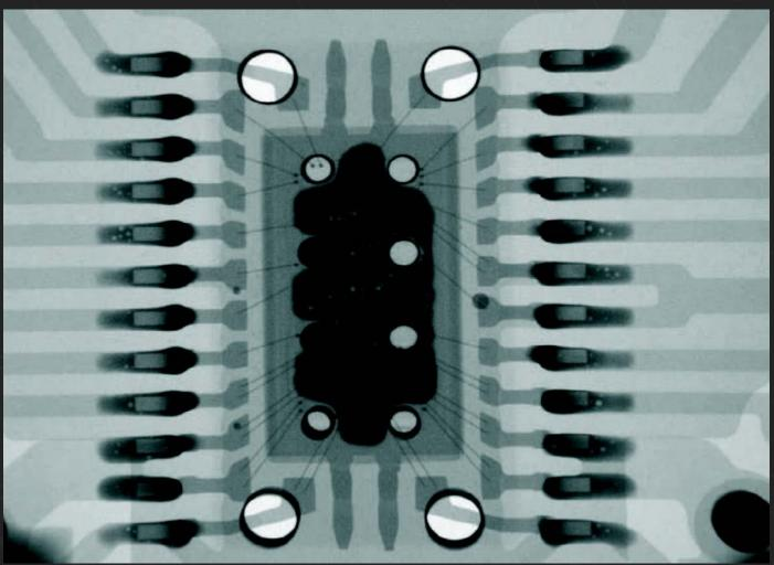
This xray image from Texas Instruments Application Note SLOA120<sup>1</sup> shows an integrated circuit with eight thermal vias used to conduct heat out of the powerpad and into the inner layers of the printed circuit board. Two of the eight vias filled with solder, contributing to solder loss across the pad and reduced thermal transfer performance of the part.
