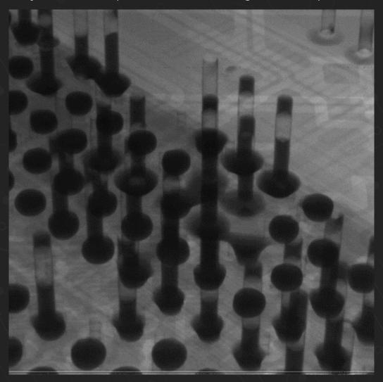
This X-Ray image shows vias in pads in a Ball Grid Array Device. The board was soldered part-side-up and is shown part-side-down, with the BGA part beneath the vias in this image. Once the solder enters a liquid phase, cohesive forces and gravity combine to draw the liquid solder into the via cavity. Without an adequate amount of solder at the surface, the copper pads on the PCB will not properly bond to the BGA pads.
