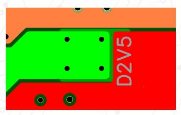
This image shows an internal power plane layer of a PCB design. The copper-pour, shown in bright green, connects net D2V5 to a different layer that is partially visible in a darker green color, with four 14-mil vias. Any heat generated in the vias will be quickly transmitted to the copper pours so the temperature of the vias will closely track the temperature of the copper above and below the vias.
