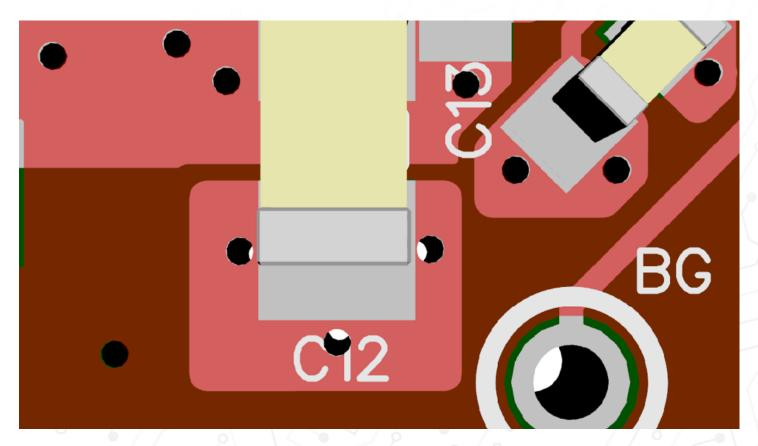
Copper vias placed very close to a pad can fill with solder during the reflow cycle. In this image, C12 has unfilled vias immediately next to the pad. The LPI solder mask may not be large enough to form a barrier between the pad and the via cavity. Fortunately, passives can be easily reworked, but BGAs, QFNs, and other leadless packages are difficult to repair.
