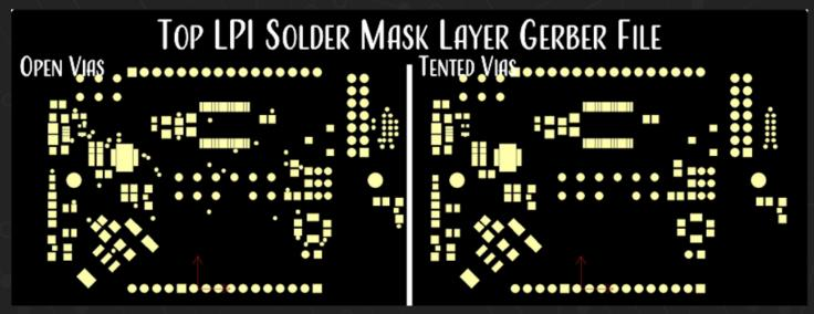
You also can ask your printed circuit board fabrication house to edit your solder mask layer to include via-tents when you submit your design files. Communicate to your fabricator via a pdf README that accompanies your Gerber 274x or ODB++ design files.
