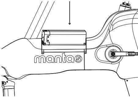
9. Perform a function check - ensure battery is off, turn pedals two full rotations and feel resistance. ⚠️ **WARNING: Do not connect the battery without ensuring that the battery is off.**
