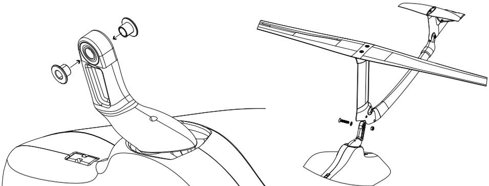
5. Rotate Hydrofoiler into upright position.
