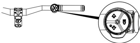
1. Bring within 1 m (3 ft) of the Hydrofoiler. Turn battery on.
