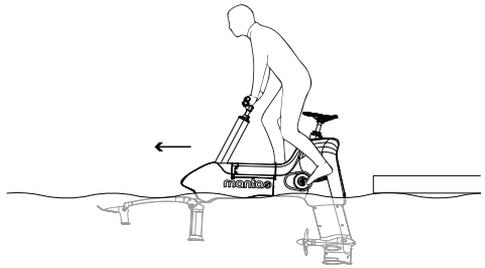
1. Place Hydrofoiler into the water at jetty edge.
