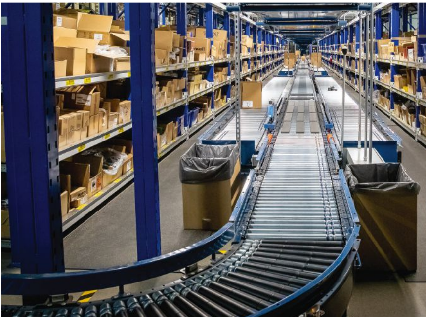
In BlueStar’s warehouse, a conveyor system brings boxes directly to employee pick stations.
