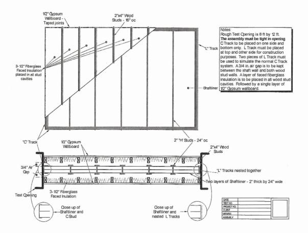
B3451-1W: Drawing received from client of wall assembly to be built
