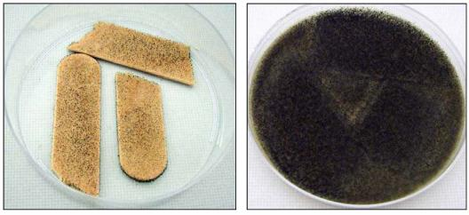
The picture on the left is of the sterile tongue blade control at Day 28 which was inoculated with the test inoculum. The picture on the right is of the sterile paper strips at Day 28 that were placed on the agar surface and inoculated with the test inoculum. Both inoculum controls verify that the test inoculum was appropriate and viable.
