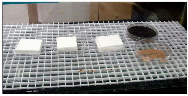
Pictured above are the three replicates tested of sample 1.2" Poly Max 9.4pcf (100% Polyester Acoustic Panel) and the test controls in the test chamber at Day 21.
