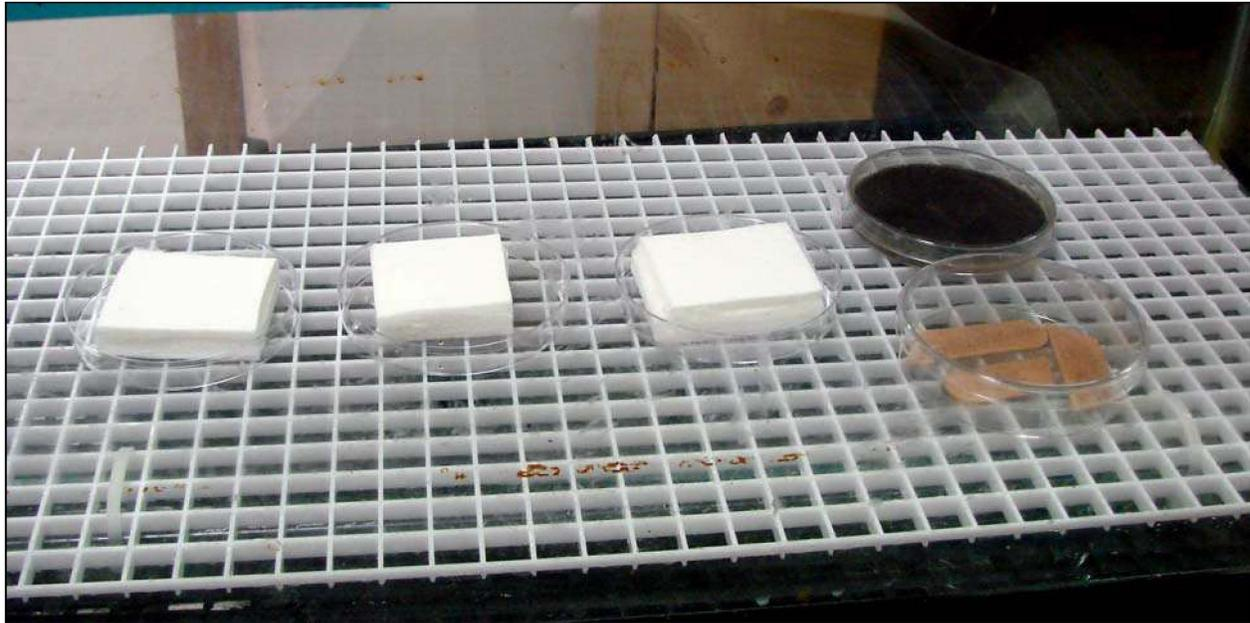
Pictured above are the three replicates tested of sample 12" Poly Max 9.4pcf (100% Polyester Acoustic Panel) and the test controls in the test chamber at Day 21.
