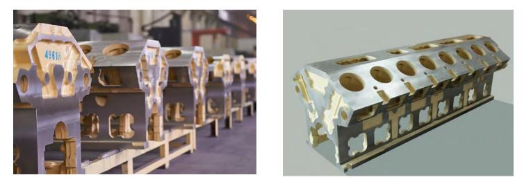
Sand casting is another ancient form of casting during which the caster creates a mold by compacting sand around a three-dimensional pattern or model of the final component. The compacted mold is then split apart, and the interior pattern is removed. The manufacturer then joins the two parts of the mold back together and pours molten metal into the cavity. Once the molten metal cools and solidifies, the sand is removed, revealing the newly cast metal part.
