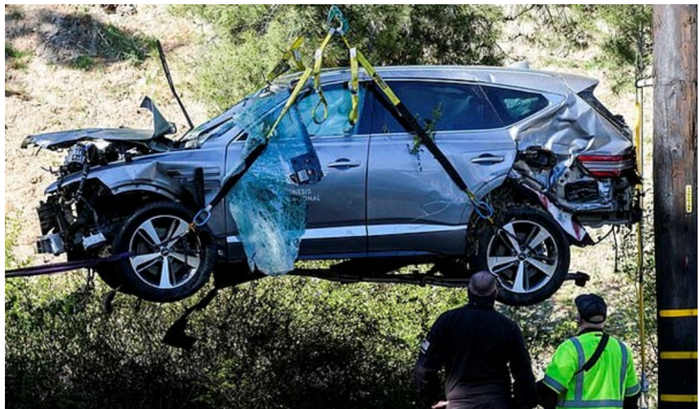
Figure 3: View showing Tiger Woods' rolled Genesis with an intact occupant compartment, intact side glazing and deployed side curtain airbags.
