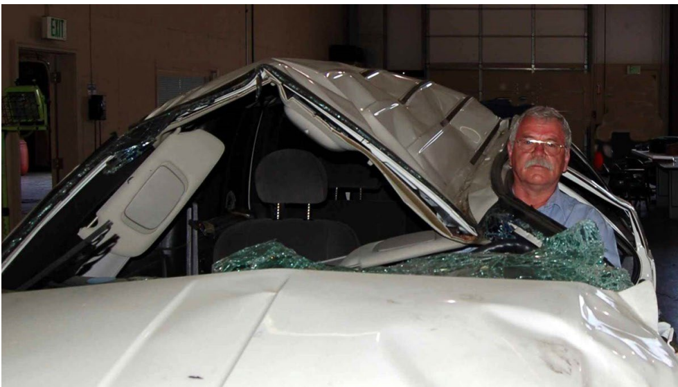
Figure 1: Raphael Grzebieta, PhD, seated in a rolled SUV that met the US roof crush design rule with a narrow margin, demonstrating a typical level of roof crush experienced in a rollover often leading to ejection of seatbelted occupants (vehicles manufactured prior to 2009 after which new regulations were enacted).
