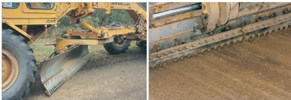
Figure E 6: Blade with grader bits
