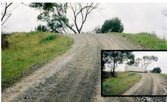
Drivers may not be aware that just over the rise there is an intersection (see inset)
