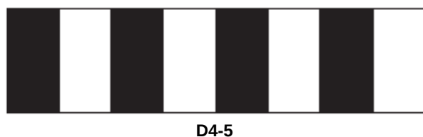
Figure B 5: Obstruction markers
