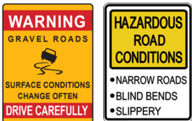
Figure B 10: Examples of non-standard warning signs for unsealed roads that can provide more specific guidance and/or advice for drivers than existing standard signs.
