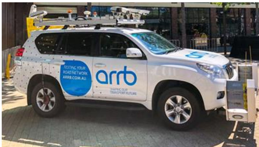
Figure 2.9: ARRB network survey vehicle
