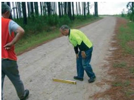
Figure 4.13: Use of a smart level with digital readout of crossfall
