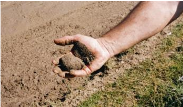
Figure 4.17: Simple field test for moisture content
