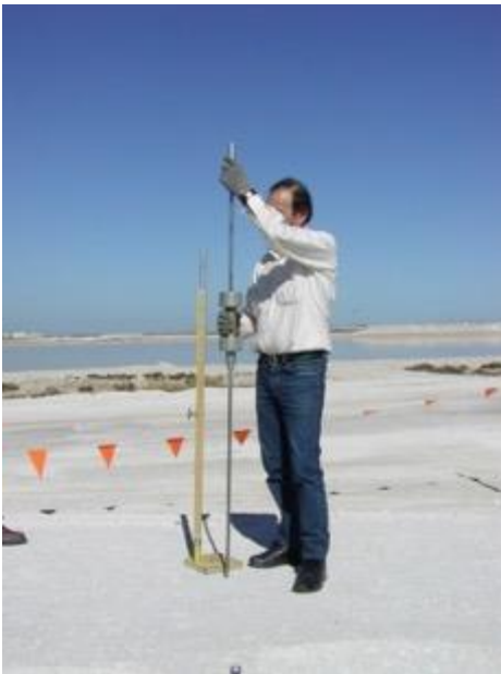
Figure 3.15: Use of a dynamic cone penetrometer
