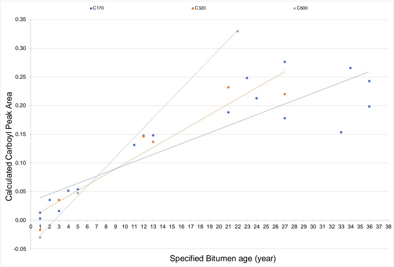
Figure 2.3 Developed FTIR reference curves for different binder types from stored samples
